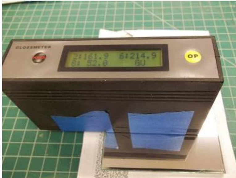
Photo No. 9 Typical Gloss Reading Test Setup Detail
