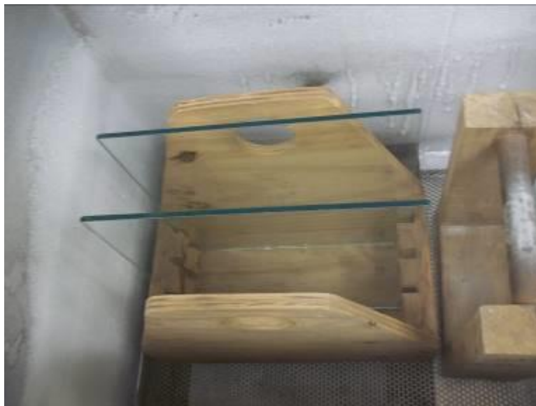
Photo No. 12 Test 28 - Resistance to Temperature Specimens Conditioning
