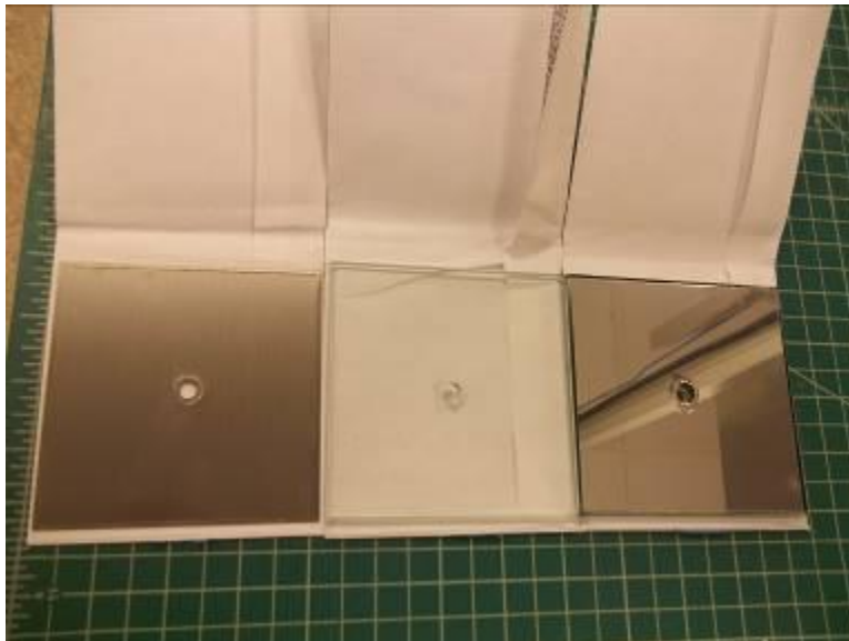
Photo No. 2 Test 17 - Specimens One of Each Shown, Left to Right, 20g Metal, Glass, and Mirror
