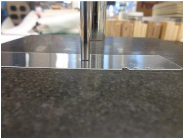
Photo No. 8 ASTM D3652 Thickness Reading
