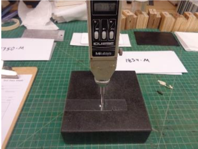
Photo No. 7 ASTM D3652 Thickness Setup
