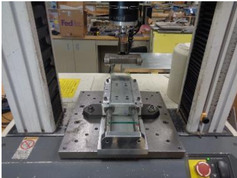
Photo No. 2 ASTM D3330 Test Setup
