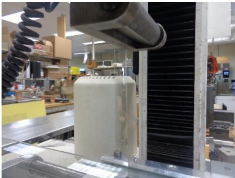
Photo No. 4 ASTM D3330 Test in Progress
